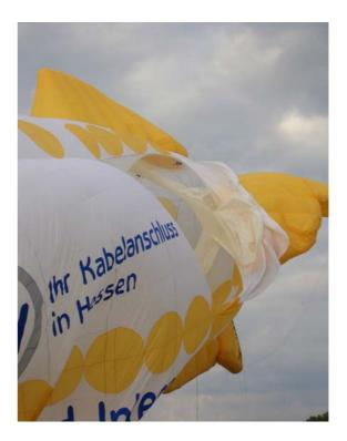
The ventilation hose was torn open along the seam to the left-hand fin over a length of more than 2 meters.
