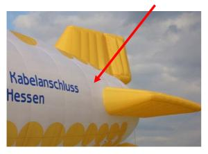
The vertical rip involving seven panels was located in the section in which the left-hand fin was incorporated. The horizontal rip was above the lefthand fin. Both rips ran along the load tapes. The seams themselves were intact.
