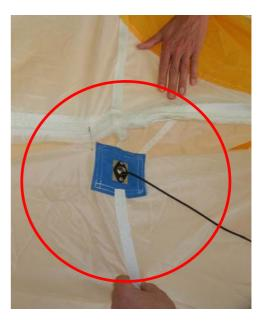
The actual positions of the eyelets in the load tape were less than optimal in view of the loads which occur in service. The load tape did not form a closed loop around the envelope but had gaps at each of the four eyelets for control lines.
