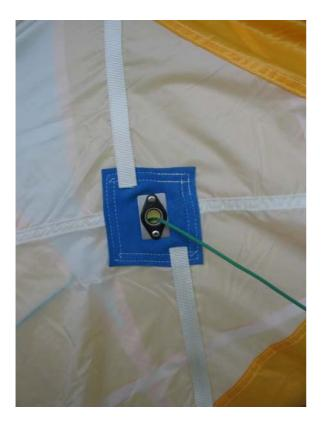
Because the envelope expanded due to the internal pressure but the load tape running around the envelope did not a very high tensile stress occurred in the area of the eyelets of the discontinuous circumferential load tapes and this caused the fabric to tear. On other eyelets, the fabric showed clear signs of high tensile stress in the run-up to tearing.
