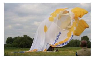
The envelope had burst open vertically and horizontally on the left-hand side in the area of the empennage involving several panels. In addition the internal left ventilation hose was torn open. A large triangular opening had formed at the tail of the airship and within a short time volume and buoyancy of the envelope decreased considerably. There was no damage to persons or property beyond the severe damage to the aircraft.
